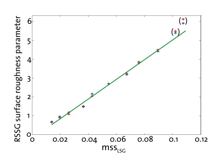
Comparison of the RSSG surface roughness parameter to mean square slope measured with a laser slope gauge [4]. Data from experiment at Marseille wind-wave facility (red and blue crosses from different days).
