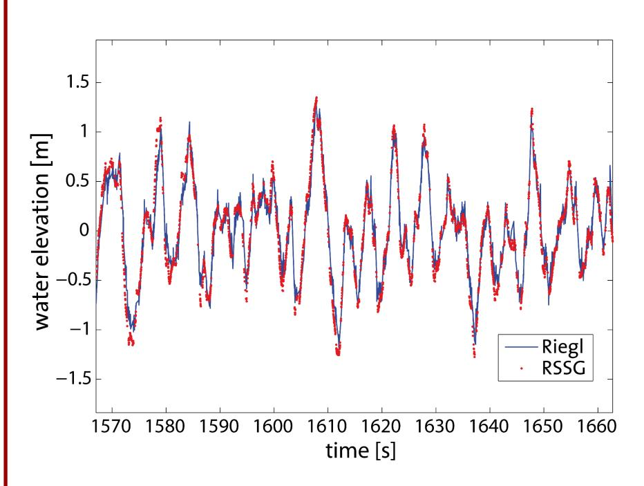
Comparison of Riegl laser altimeter (blue line) and surface elevation from stereo with the RSSG (red dots) during the OSSPRE cruise on R/V Kilo Moana.
