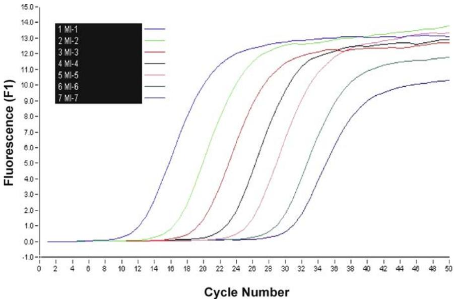
**Fig. 1** Quantitative real-time amplification plot of a representative standard curve (tenfold dilutions of a plasmid). The insert graph is a plot of the Ct values vs the log of the concentration where the slope of the curve is  $-3.386$
