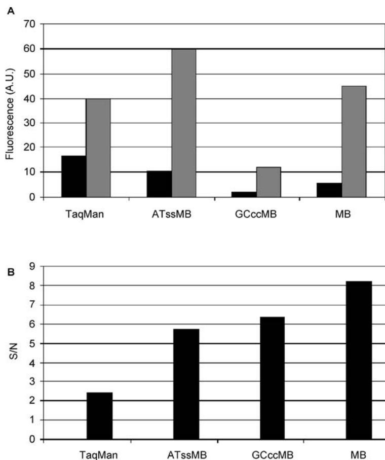
**Fig. 4** **A** Fluorescence signals after completion of PCR (*gray columns*) for various real-time PCR probes. The black columns show the initial fluorescence background averaged over the first five PCR cycles. AU, arbitrary units. **B** Signal-to-background ratios ( $S/N$ ) obtained using the data given in **A** for the four real-time PCR probes
