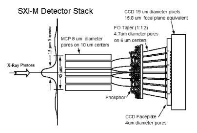
Figure 3. Detector stack schematic (Bornmann et al., 1997).
