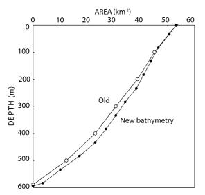
Fig. 7 Area versus depth for Crater Lake from new bathymetry from Gardner and Dartnell (2001) and old bathymetry from Byrne (1965). Note that lake area and volume given in Byrne (1965, Table 1) are not correct for his map
