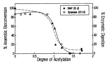
Fig. 7. Comparison of anaerobic biodegradaton and enzymatic hydrolysis for the xylan acetate polymer series. Data for BMP analysis represent the average of triplicate experimentals. Data for xylanase hydrolysis represent the average of duplicate determinations.
