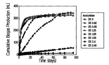
Fig. 3. Anaerobic biodegradation of cellulose acetate polymers of different degrees of acetylation. The BMP assay was performed as described in the Materials and Methods section.
