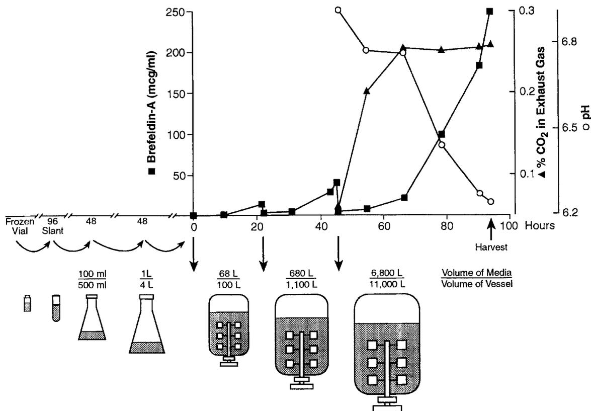
Figure 2 Scheme for scale-up production of brefeldin-A to an 11000-L fermentor providing a time line and volume at each stage
