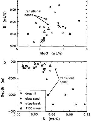
Fig. 7. a Plot of S vs MgO showing the range of S contents and that S content is not related to composition. b Plot of depth vs S content showing that lavas recovered shallower than about 1600 m contain < 0.07 wt.% S whereas those recovered deeper than 1600 m contain >0.05 wt.% S. See text for discussion
