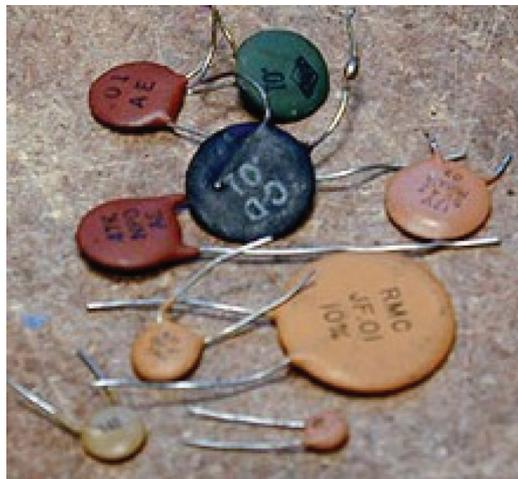
Figure 4. Examples of early ceramic capacitors taken from antique radios. Early ceramic capacitors looked very much like modern examples, although somewhat larger for a given capacitance. Then, as now, ceramic capacitors were very reliable. Photo courtesy of P. I. Nelson, [www.antiqueradio.org](http://www.antiqueradio.org), and used with permission.
