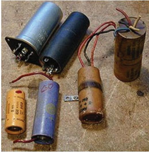
Figure 3. Examples of early electrolytic capacitors taken from antique radios. These capacitors are also unreliable and are replaced when restoring such a radio. Photo courtesy of P. I. Nelson, [www.antiqueradio.org](http://www.antiqueradio.org), and used with permission.
