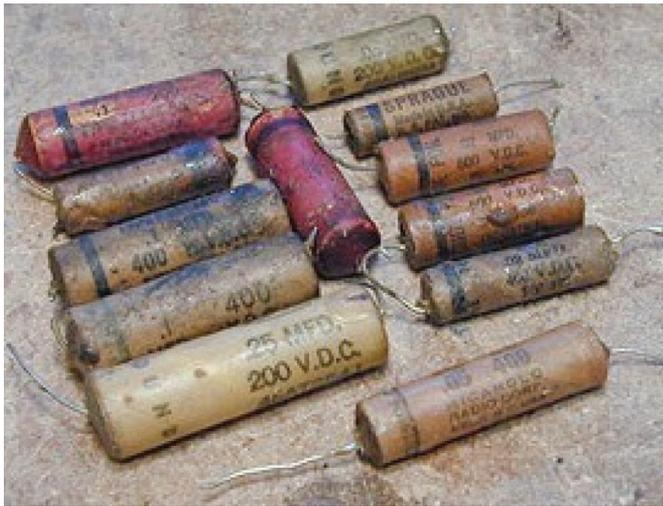
Figure 1. Examples of early waxed paper and foil capacitors taken from antique radios. Such capacitors tend to be unreliable and are usually replaced with metalized polymer film capacitors when restoring a radio. Photo courtesy of P. I. Nelson, [www.antiqradio.org](http://www.antiqradio.org), and used with permission.
