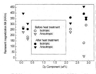
Fig.2. Measured remanent magnetization M<sub>r</sub> of NdFeB materials versus Dy component.
