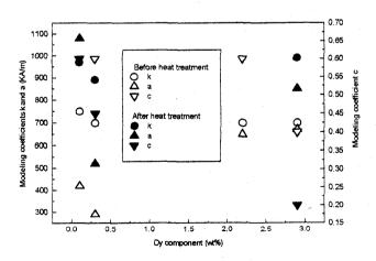
Fig.5. Modeling coefficient versus Dy component of NdFeB materials
