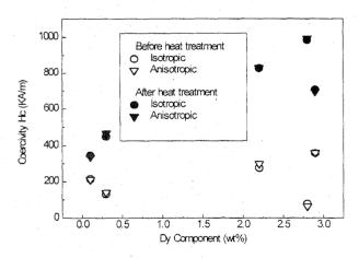
Fig.1. Measured coercivities  $\rm H_{c}$  of NdFeB materials versus Dy component.
