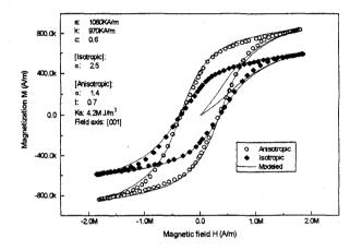
Fig.4. Modeled and measured hysteresis curves of sample 1 after heat treatment
