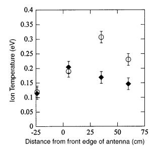
FIG. 5. Perpendicular ion temperatures in HELIXa at different axial locations for a magnetic field strength of ( $\blacklozenge$ ) 453 G and ( $\bigcirc$ ) 808 G.
