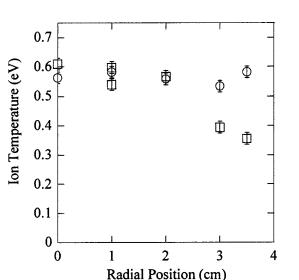
FIG. 4. ( $\bigcirc$ ) Perpendicular and ( $\Box$ ) parallel ion temperatures vs radius for a fill pressure of 6.7 mTorr and a rf power of 750 W for a rf frequency of 9 MHz.
