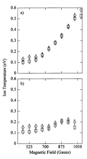
FIG. 3. (a) On axis  $(\bigcirc)$  perpendicular and  $(\square)$  parallel ion temperature as a function of magnetic field strength for HELIXb in the eight-coil configuration at position "B" with a fill pressure of 6.7 mTorr, and 750 W of rf power for (a) a rf frequency of 9 MHz and (b) a rf frequency of 13.5 MHz.
