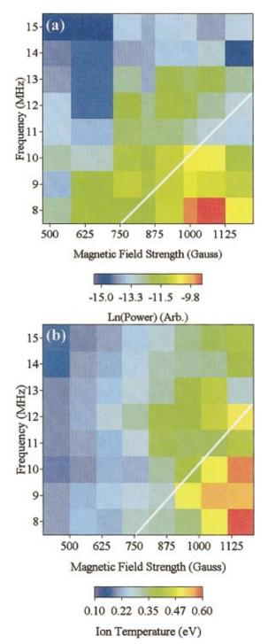
FIG. 9. (Color) (a) Signal amplitude of the low frequency wave at location "B" and (b) perpendicular ion temperatures at location "A" with HELIXb in the eight-coil configuration for a fill pressure of 6.7 mTorr and a rf power of 750 W.
