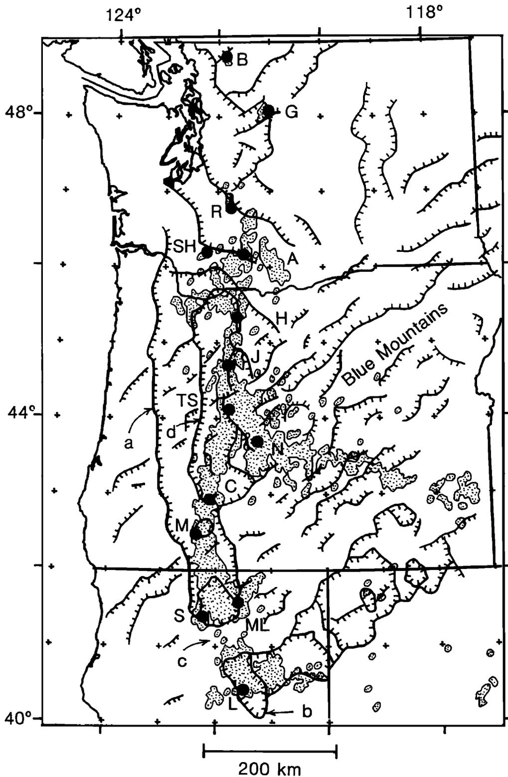
Fig. 4. Interpretation of boundary analysis. Bold, hachured lines indicate boundaries between regions of disparate density as interpreted from Plate 1 and Figure 2; hachures point toward less dense areas. Stippled area indicates lateral extent of Pliocene and Quaternary vents (Figure 3). Capital letters and associated dots are major volcanoes; see Figure 1 for volcano names. Lowercase letters indicate features discussed in text.
