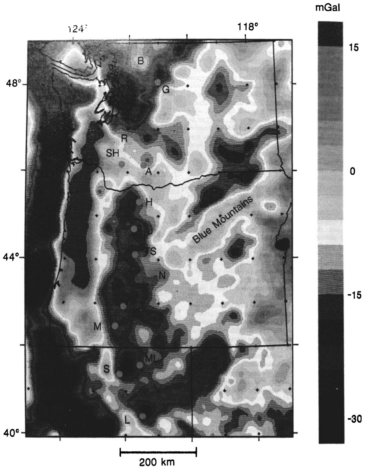
Plate 1. Isostatic residual gravity continued upward 10 km. Color contour interval 3 mGal. Dots indicate major volcanoes; see Figure 1 for definition of labels.
