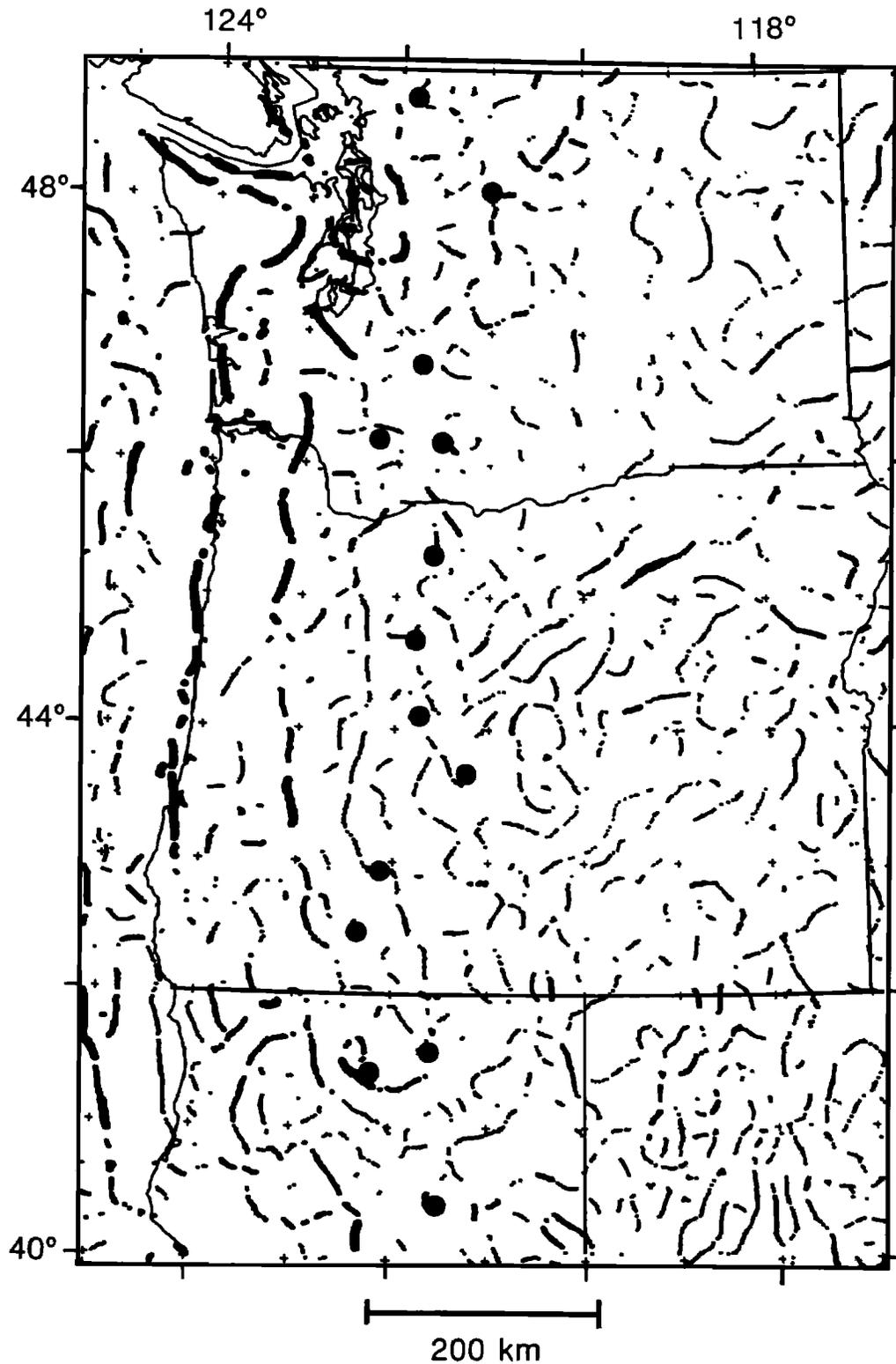
Fig. 2. Automatically calculated boundaries between mass densities. Size of dot represents steepness of horizontal gradient. Smallest dot, 0.2–0.5 mGal/km; medium-sized dot, 0.5–1.0 mGal/km; largest dot, >1.0 mGal/km. Very large dots indicate major volcanoes; see Figure 1 for labels.
