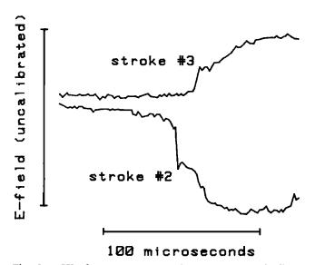
Fig. 2. NSSL fast antenna recording system electric-field waveforms (uncalibrated) of the second and third strokes in the triggered flash of Figure 1. The 10-90% risetime of the fast antenna was  $0.5 \ \mu s$  with a decay time of 1 ms.
