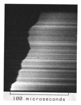
Fig. 1b. Time-resolved streak photograph of the third stroke of the triggered flash shown in Figure 1a. A #29 deep red filter was used during imaging to minimize background exposure.
