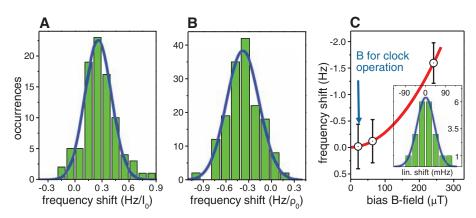
**Fig. 3.** Clock shift sensitivities. Histogram of clock shift sensitivity to (**A**) the lattice laser intensity slightly away from the magic frequency and (**B**) the atomic density. (**C**) One of 20 data sets indicating the clock sensitivity to magnetic fields. The inset to (C) shows the histogram of the linear Zeeman shift evaluated at  $B_{0}$ , based on the 20 data sets.
