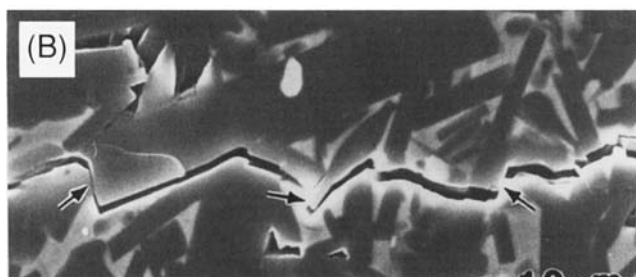
Fig. 1. SEM views of cracks in (A) homogeneous control and (B) heterogeneous test SiC. Note relatively straight, transgranular path in (A), and bridged, intergranular path in (B). (After Ref. 1.)
