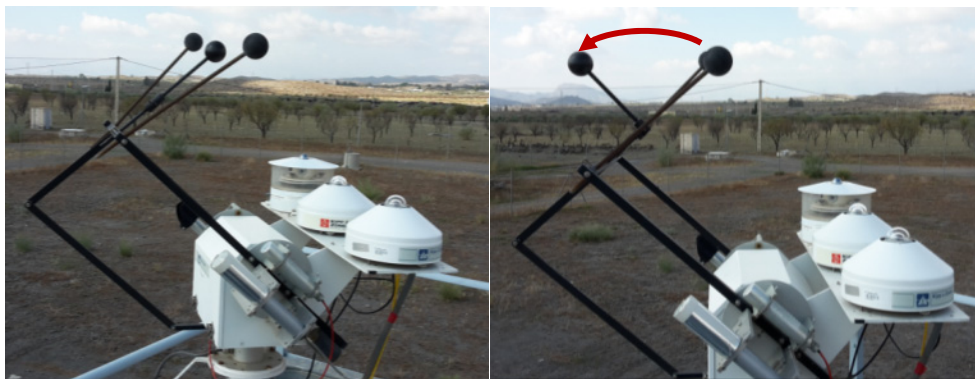
Figure 6. 2AP sun tracker with modified shadow structure for alternating sun-and-shade method: Left: shadow ball in shade position over reference pyranometer (DHI measurement). Right: shadow ball in sun position reference pyranometer free from shade (GHI measurement).
