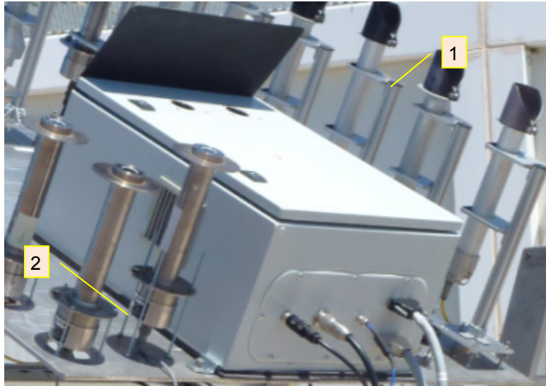
Figure 4. Mounting structure for field pyrhelimeters: 1) support structure for Kipp&Zonen, Hukseflux and Eko pyrhelimeters and 2) Eppley NIPs mounted via three threaded rods.
