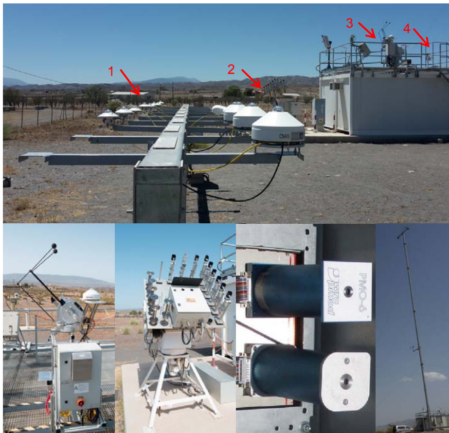
Figure 1. Top) Overview of Metas calibration setup (1: Pyranometer test bench; 2: Pyrheliometers test bench; 3: Black Photon tracker with DHI reference; 4: cloud camera); Bottom left) detail view of Black Photon tracker; Bottom left centre) detail view of pyrheliometer test bench; Bottom right centre) two absolute cavity reference pyrheliometers located at pyrheliometer test benchfront cabinet; Bottom right) Metas wind mast.
