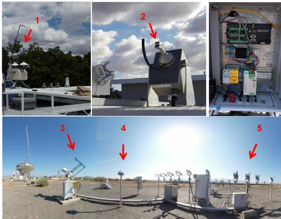
Figure 2. Top left) Madrid calibration setup (1: Tracker with reference sensors and 2: mounted RSI); Top right) Data acquisition system used in Madrid setup; bottom) PSA test setup (3: Tracker with reference DNI and DHI measurement, 4: GHI measurement for quality check of reference data and 5: RSI test bench)
