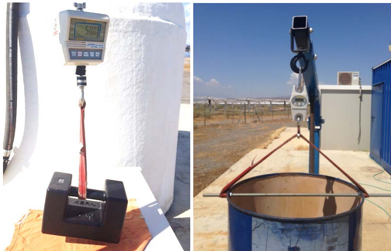
Figure 12: left: calibration of the crane weigher using a 50kg class M2 ( \pm 8 g) weight (loop tared) right: measurement setup, empty barrel (tared) at the crane weigher
