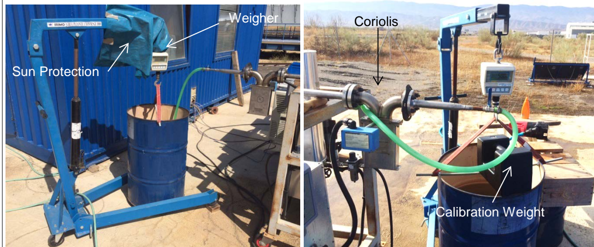
Figure 13: left: setup during measurement right: linearity check, calibration weight on top of filled barrel
