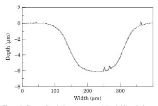
Figure 2. Shape of typical crater sputtered in obsidian during a SIMS analysis. Only ions from the centre  $\sim 30 \,\mu\text{m}$  of the crater (flat area) are analysed. Note  $\sim 40:1$  vertical exaggeration.
