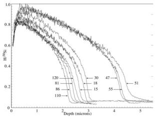
Figure 6. Summary of hydrogen depth profiles in all samples. Profiles are labelled using abbreviated sample numbers (no CHO).
