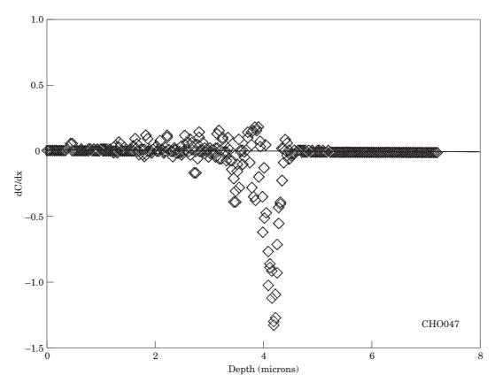
Figure 9. The first derivative of the concentration as a function of depth for sample CHO047. The inflection point is located at the minimum of the negative spike near 4 µm depth.
