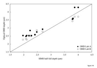
Figure 14. Plot of half-fall depth measured using SIMS against the "half-fall" depth measured using optical techniques in two different laboratories. Stated errors are smaller than the symbol size.
