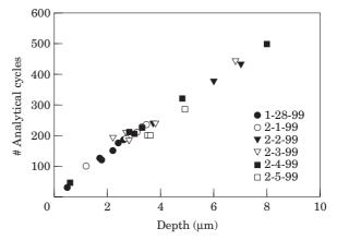
Figure 3. Plot of crater depth as a function of number of analytical cycles on Pachuca obsidian. Data obtained over a 2 week period. All analyses conducted using a 130 nA primary ion beam rastered over a  $150 \times 150 \ \mu\text{m}^2$  area. Analytical cycles are directly correlated to time of sputtering (100 cycles ~45 min).
