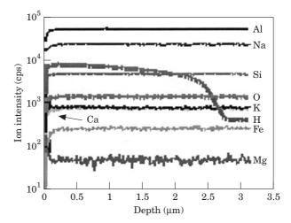
Figure 5. Profile illustrating the variation in ion intensities (directly correlated to concentration) as a function of depth in a typical profile (CHO120).
