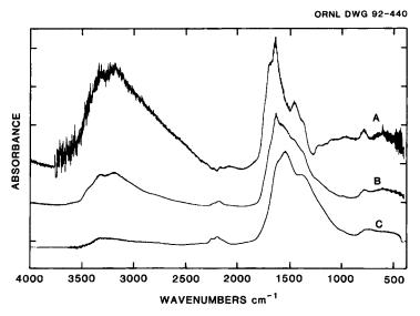
**Figure 2.** Infrared spectra of: (A) difference (B-C), (B) paracyanogen film on silicon after 3 months exposure to air, (C) freshly sputtered film of paracyanogen on silicon.
