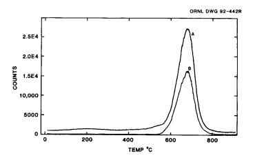
Figure 3. Mass analyzer response: (A) profile of total ion current versus temperature in the decomposition of paracyanogen derived from silver cyanide (product A), (B) ion of mass 52.
