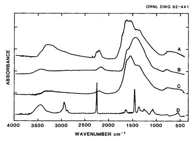
Figure 1. Infrared spectra of: (A) photochemical product dispersed in KBr, (B) chemical product derived from AgCN, (C) sputtered product on silicon wafer, (D) polyacrylonitrile in KBr pellet.
