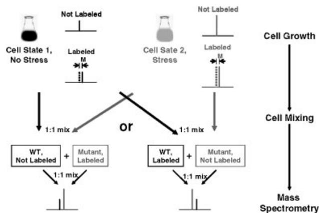
**Scheme 1.** Scheme for the strategy of stable isotope assisted mass spectrometry for accurate quantitation of protein expression levels in two different cell populations. Stress can be radiation, heat shock, mutation of the same cell and others in different studies.
