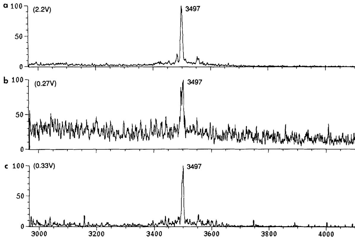
**Figure 1** (a) Mass spectrum from 5 ng of oxidized insulin B-chain acquired by coaxial continuous flow FAB. (b) Mass spectrum from 5 ng of oxidized insulin B-chain acquired by static FAB. (c) Single-scan mass spectrum of 0.7 ng of oxidized insulin B-chain acquired by coaxial continuous flow FAB.
