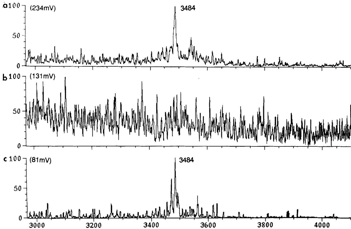
**Figure 2** (a) Mass spectrum from 5 ng of glucagon acquired by coaxial continuous flow FAB. (b) Mass spectrum from 5 ng of glucagon acquired by static FAB. (c) Single-scan mass spectrum of 0.7 ng of glucagon acquired by coaxial continuous flow FAB.
