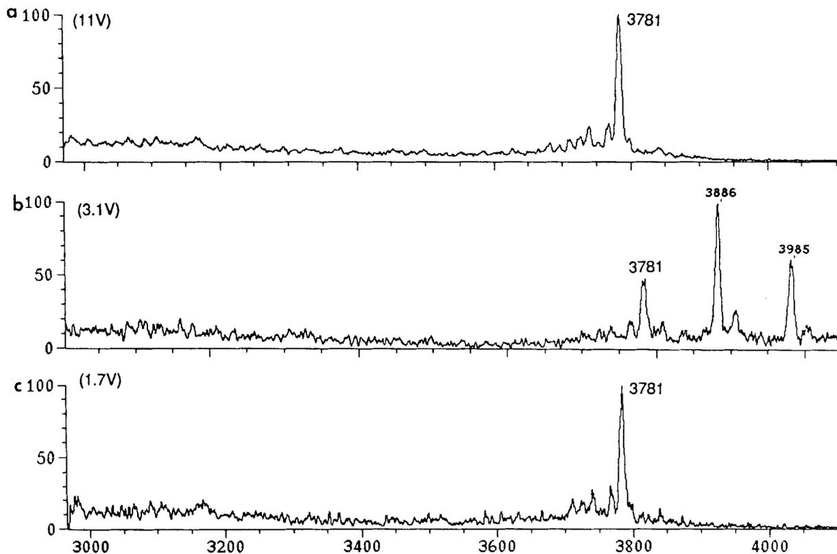
**Figure 4.** (a) Mass spectrum from 100 ng of Tyr-C-peptide acquired by coaxial continuous flow FAB. (b) Mass spectrum from 100 ng of Tyr-C-peptide acquired by static FAB. (c) Single-scan mass spectrum of 14.4 ng of Tyr-C-peptide acquired by coaxial continuous flow FAB.
