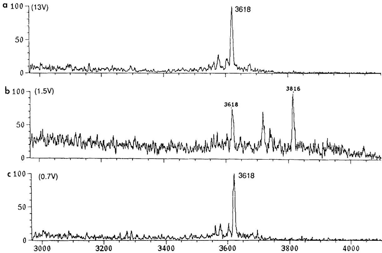
**Figure 3.** (a) Mass spectrum from 29 ng of C-peptide acquired by coaxial continuous flow FAB. (b) Mass spectrum from 25 ng of C-peptide acquired by static FAB. (c) Single-scan mass spectrum of 1.4 ng of C-peptide acquired by coaxial continuous flow FAB.
