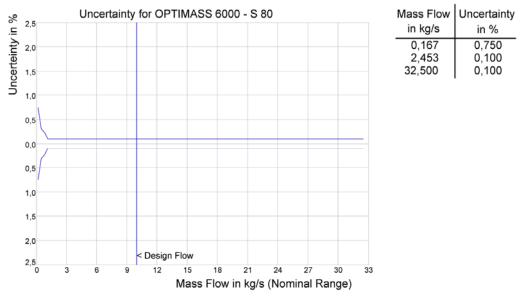
Figure 1: Measurement uncertainty over nominal mass flow for Krohne OPTIMASS 6000 - S 80 series
