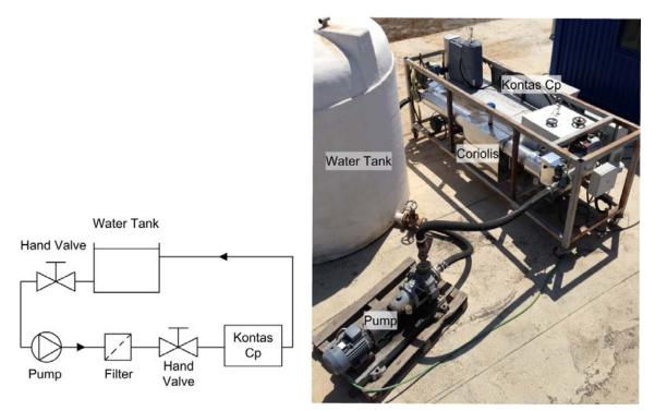
Figure 4: Water circuit with flow through measurement bypass, left: flow chart of the water circuit, right: photograph of the setup with Coriolis mass flow sensors installed
