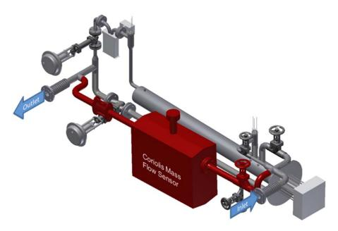
Figure 3: 3D view of the bypass facility without thermal insulation. New tube section and Coriolis sensor highlighted in red
