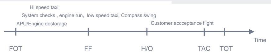
FOT: Final assembly line Operational Test FF: First Flight H/O: Hand Over TAC: Technical Aircraft Completion TOT: Transfer of Title
