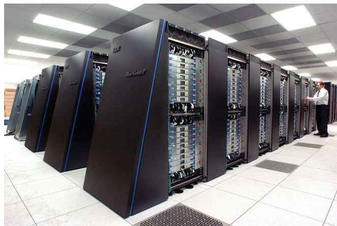
FIGURE 4.2: Example of supercomputer. In this case the model is an IBM Blue Gene/P. Note the big size of the components and the large facility. (Argonne National Laboratory. [Accessed: 05 november 2014])
