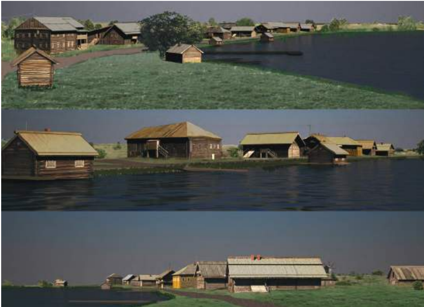
Fig. 12 A virtual reconstruction of the wooden village of Yamka on Kizhi Island, Karelia, Russia. The 3D model has been realised starting from the real dimensions obtained from the laser scanner survey. Real photomaps were used to map the buildings. This 3D model could be used for virtual navigation within an exhibition or directly on the Web.
