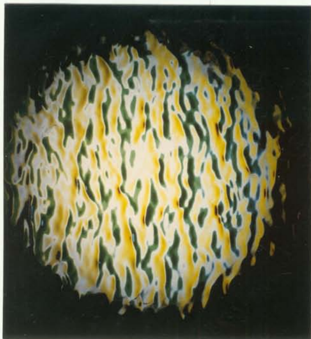
Figure 5.18: Temporal growth of the wave field in the large circular wind-wave tunnel at about 6 m/s. A sector of 20 cm in diameter is shown.
