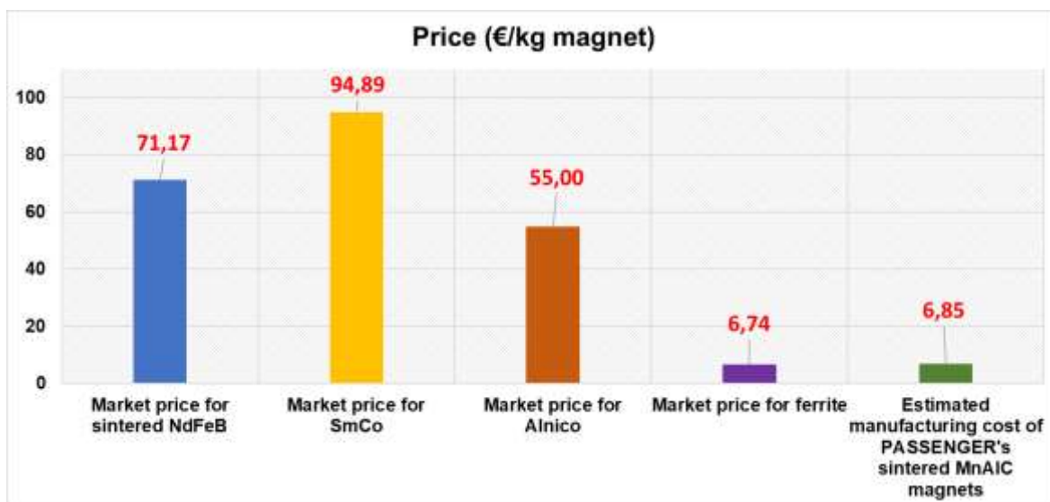
Figure 63. Comparison of the estimated manufacturing cost of 1 kg sintered MnAlC magnets with the market price of magnets containing CRMs.
