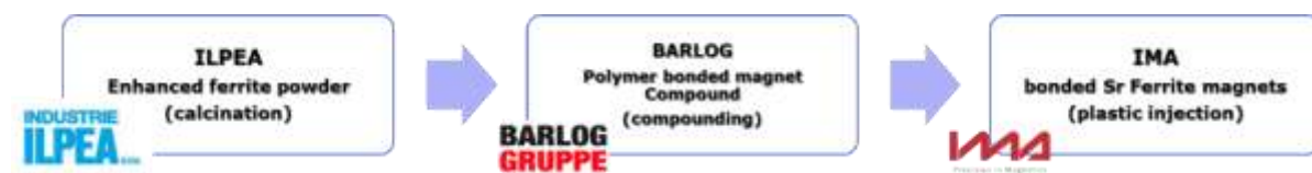
Figure 52. Production chain of PASSENGER's bonded Sr-ferrite magnets.
