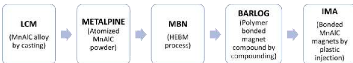
Figure 24. Production chain of PASSENGER's bonded MnAlC magnets.
