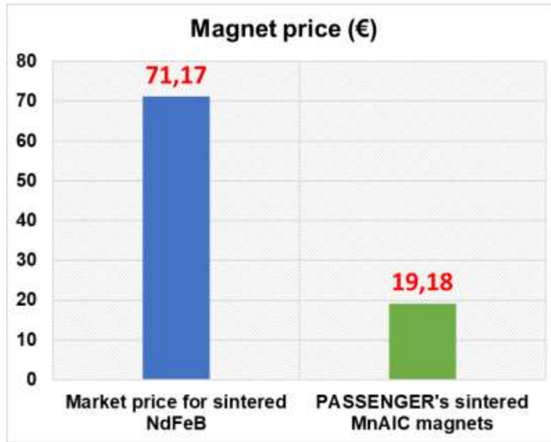
Figure 66. Comparison of the estimated manufacturing cost of sintered MnAlC magnets with the market price of sintered NdFeB permanent magnets based on magnet performance.
