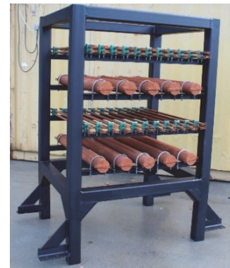
Figure 1. Steel frame and position of the eight bolts/pressure transducers (left) and pipe rack (right).
