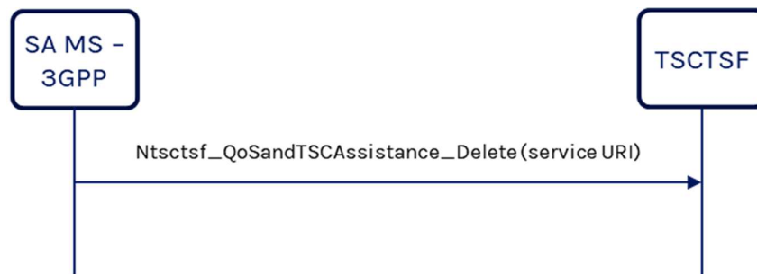
Figure 11-16 Deleting service with deterministic QoS in 3GPP domain
