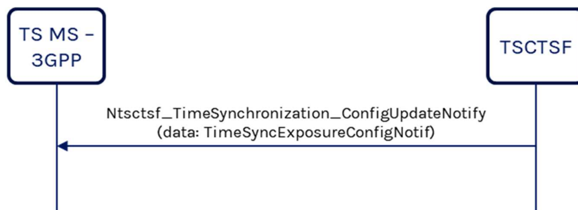
Figure 11-7 Monitoring time sync status in 3GPP
