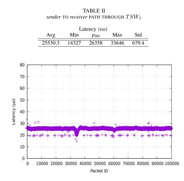
Fig. 3. Latency of the initial configuration, through  $TSW_1$  switch.
