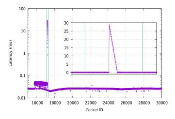
Fig. 6. Experiment 3: Time Aware Shaper on the  $TSW_1$  and zoom for a comparison with other experiments.
