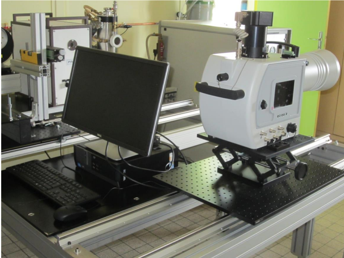
Photo n°3: Spectroradiometer SR5000N during laboratory calibration
