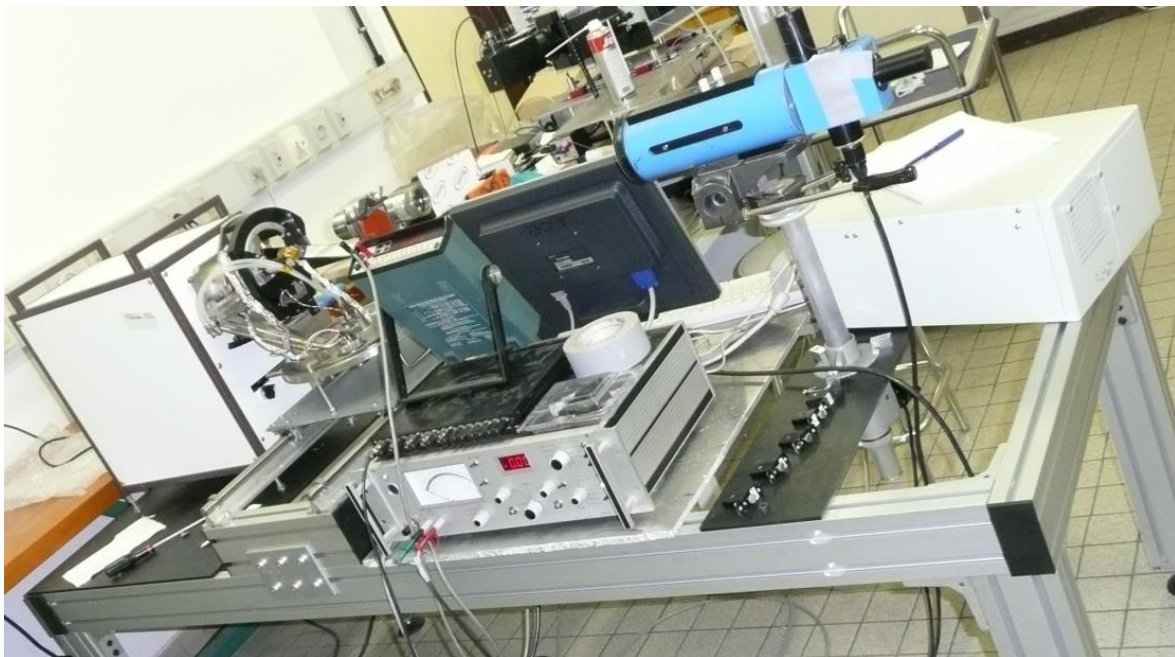
Photo n°5: calibration of the radiometer in front of a black body with the top of Mediase.
