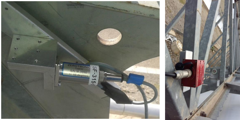
Figure 8. Right hand-WYLER Inclinometer mounted to the end-plate of a parabolic trough with a magnetic adapter. Left-hand Sensorex_sx41100 inclinometer mounted on the torque box of a parabolic trough.
