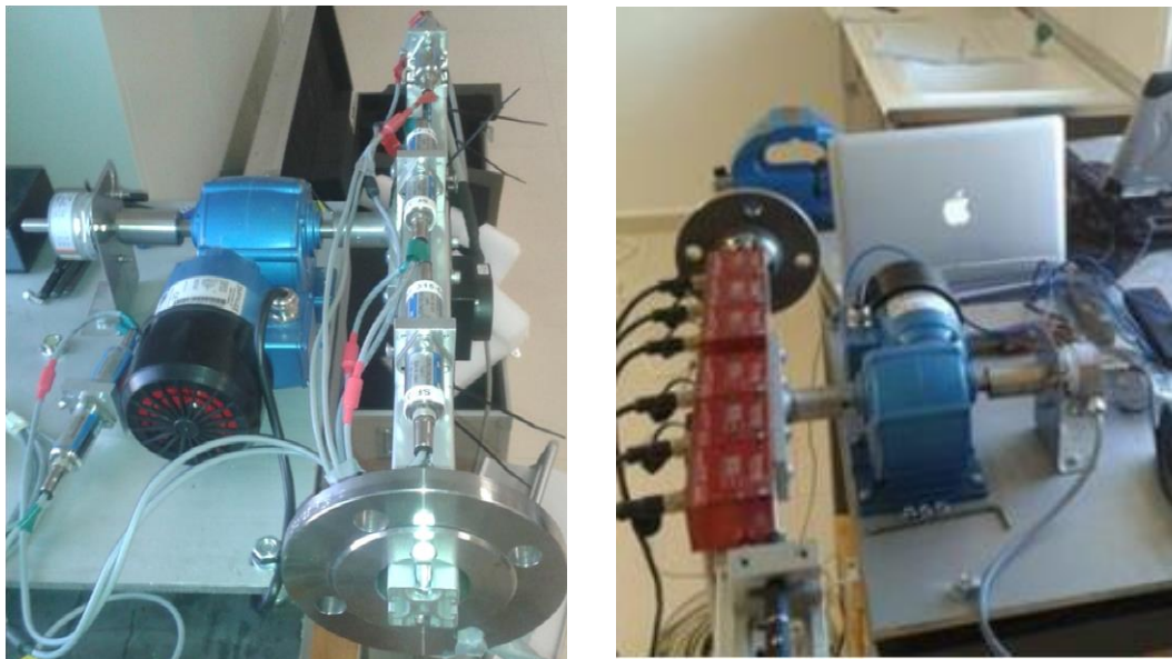
Figure 10. CIEMAT's test bench for inclinometer calibration. Right hand ZeroTronic Typ C from WYLER inclinometers and left hand Sensorex_sx41100 inclinometers being calibrated.
