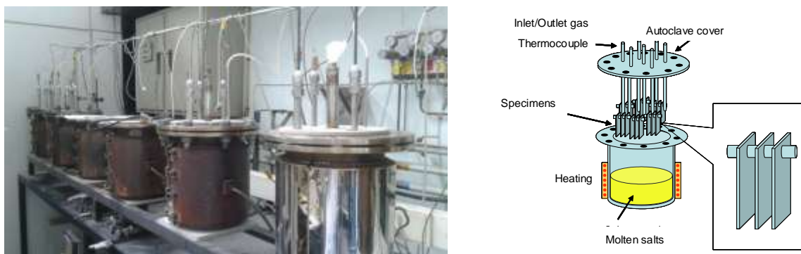
Figure 15 Autoclaves used for tests with molten salts (SMD Ciemat Laboratories)
