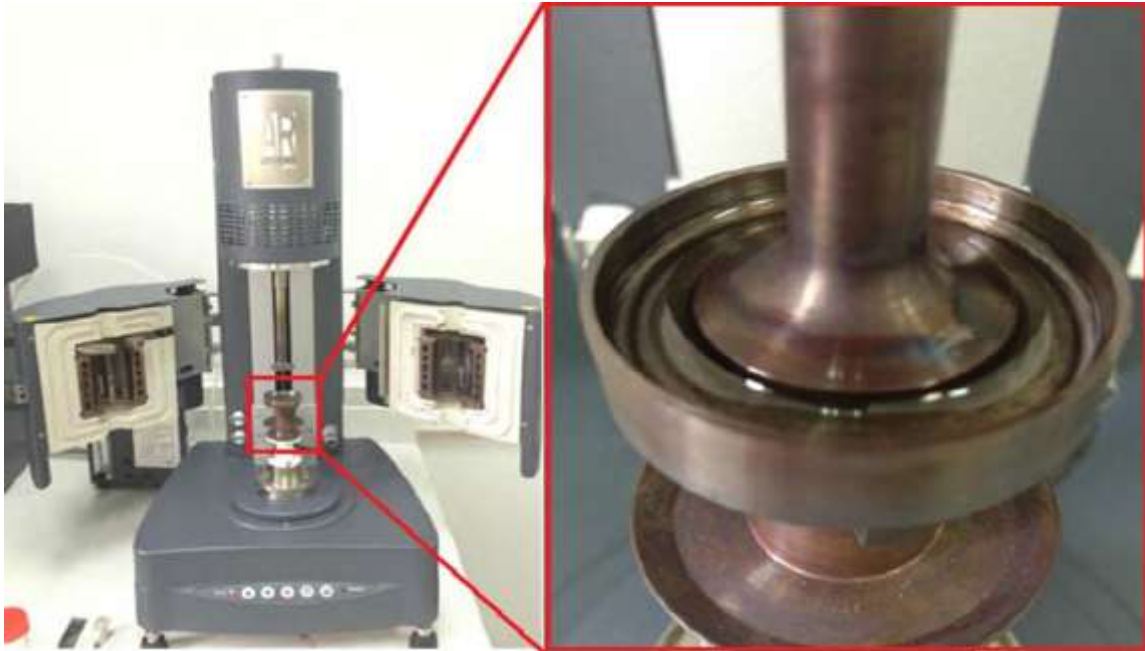
Figure 6 Rheometric system used and sample positioning for viscosity measurement
