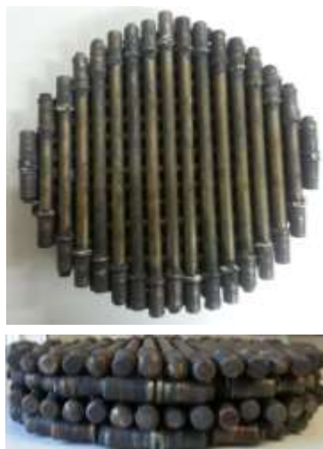
Fig. 5: Photographs of the encapsulated PCM and the arrangement in rows.
