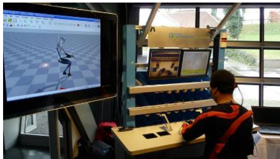
Figure 6-1: TNO assembly working cell: work instructions are presented making use of augmented reality. Working postures and movements can be measured and assessed by Xsens and Kinect.
