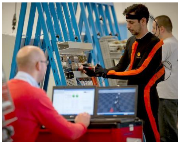
Figure 6-2: TNO Human movement and posture registration systems: Xsens and Kinect
