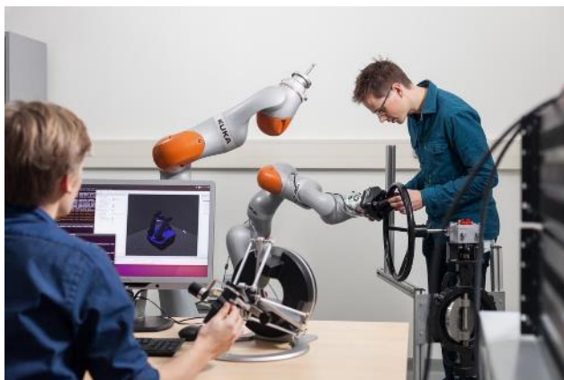
Figure 6-3: Robotic arms in TNO CC controlled by teleoperation device
