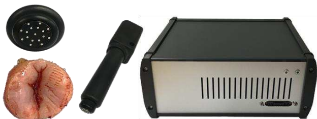
Figure 1: Impedance spectroscopy with multiple electrode probe and excised cervical tissue (normal case).
