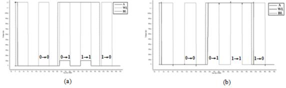
Figure 8. (a) Transient waveforms of a write failure in the traditional 5T SRAM cell, (b) Transient waveforms of a successful writing in the proposed 5T SRAM cell.
