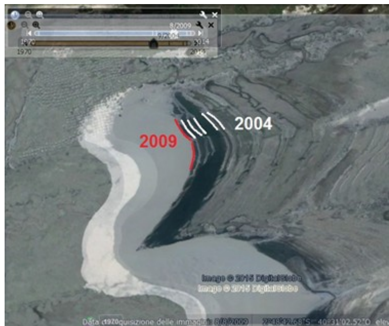
Figure 3: We can easily compare the motion of the dune, using the two images of Figure 2. In this case, we used GIMP to create an image from two layers adjusted with Retinex filtering. Red line marks the position of the toe of the dune in 2009, whereas white lines mark its position in the previous years. Note the "footprints" of the dune.
