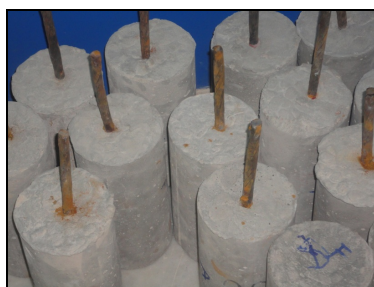
Fig. 1. Samples for pull out test
