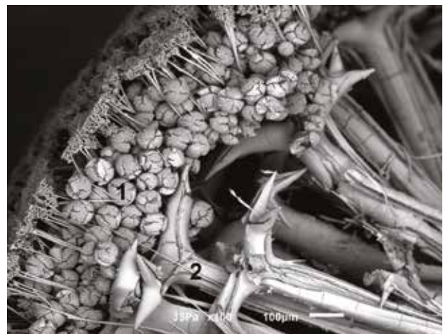
The scanning electron microscopic (SEM) observation of the bioceramics obtained after calcination (at 800°C) of deep-sea sponge, Geodia barretti (P. Tiago Henriques da Silva, University of Minho).
