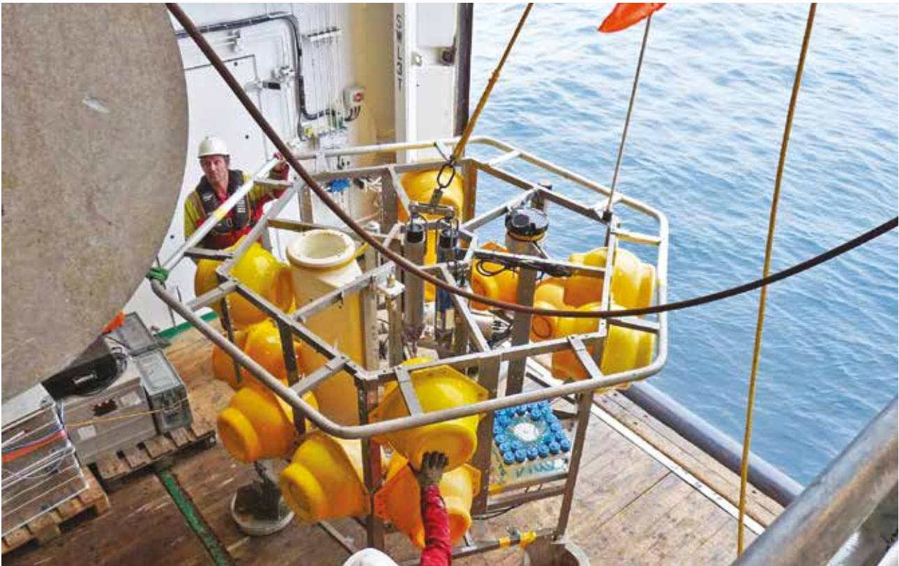
Benthic lander ready to be deployed (Photo credit: Furu Mienis, Royal Netherlands Institute for Sea Research).
