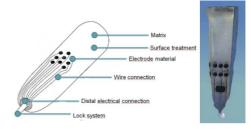
Fig. 2. First prototype of improved electrode liner for multi-channel EMG recording in transradial amputees.
