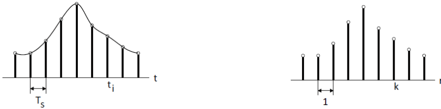
(a) A signal that is sampled to a discrete-time sequence on a time interval of T_s . Note that the axis is given as time t . (b) The discrete signal runs on a axis N for number of points. The time between one point and another is no more determinable.
