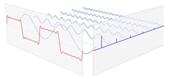
FIGURE 2.2: Dual Time-Frequency representation of the Fourier Transform (from [2])
