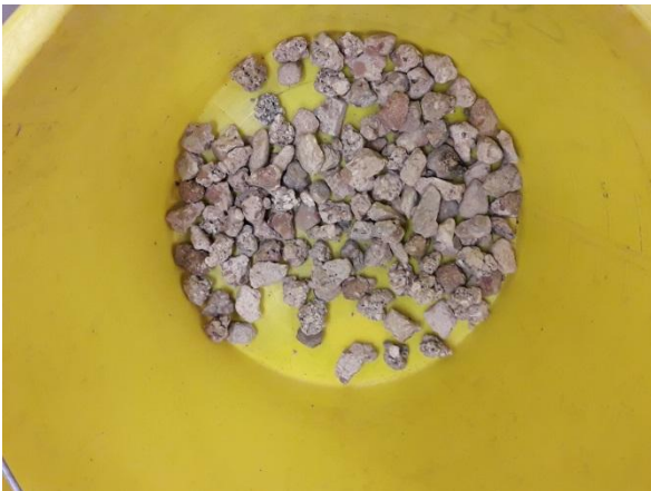
Fig. 19: Mixed concrete/mineral aggregate (16-20 mm) fraction
