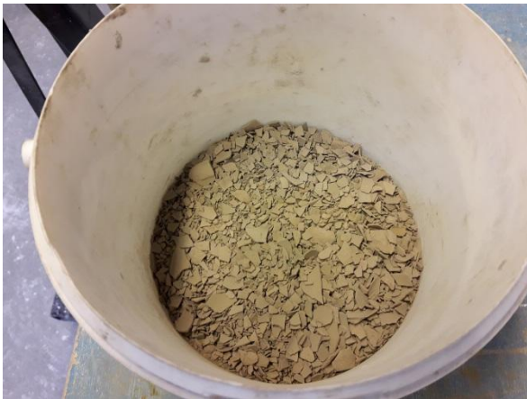
Fig. 11: Silt/clay (< 0.075 mm) sample
