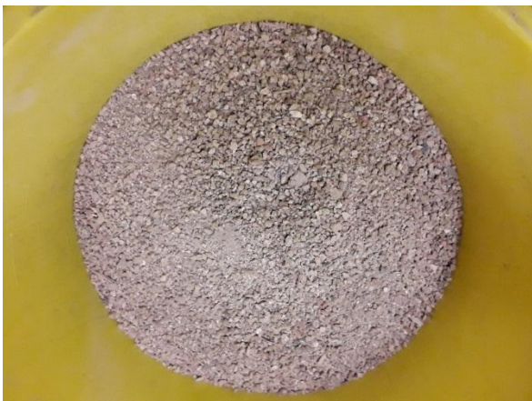
Fig. 22: Medium/coarse sand (0.6-4 mm) fraction
