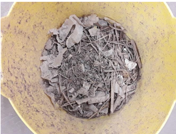
Fig. 17: Lightweight (mixed wood/plastics > 1.7 mm) fraction
