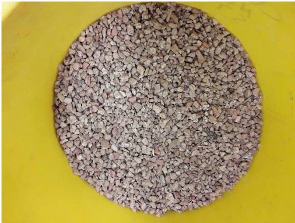
Fig. 21: Mixed concrete/mineral aggregate (4-8 mm) fraction
