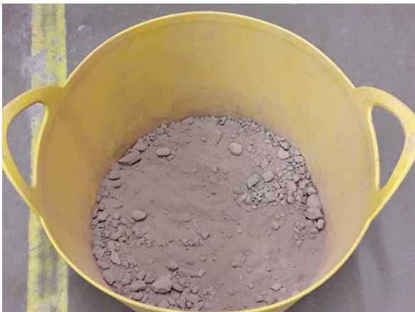
Fig. 9: Fine CDW material (< 0.6 mm)
