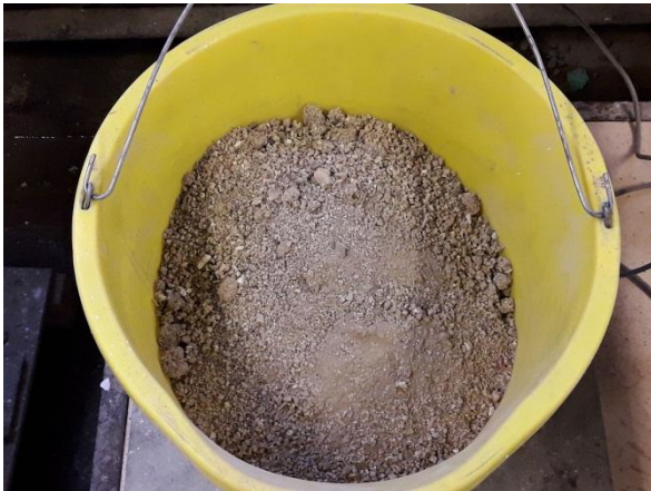
Fig. 8: Medium/coarse sand (0.6-4 mm) fraction
