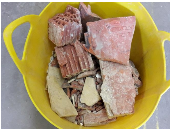
Fig. 28: Ceramics (bricks and tiles > 1.7 mm) fraction
