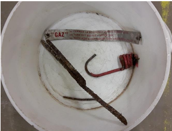
Fig 16: Steel (nails, re-bars, hooks, tags etc. > 1.7 mm) fraction
