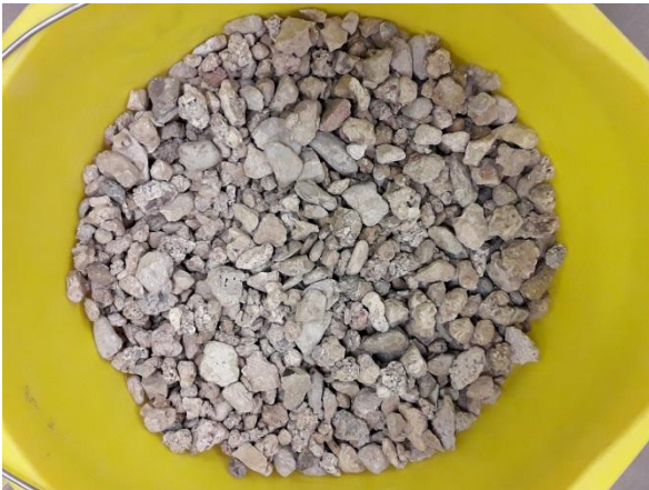
Fig. 18: Hand-picked mixed concrete/mineral aggregate (> 1.7 mm)
