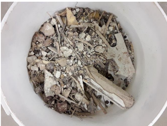
Fig. 32: Lightweight (mixed wood/plastics > 1.7 mm) fraction
