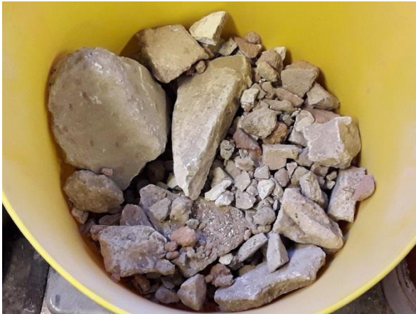
Fig. 12: Mixed concrete/mineral aggregate (> 20 mm) fraction
