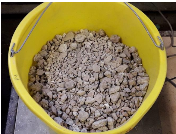
Fig. 4: Hand-picked mixed concrete/mineral aggregate (> 1.7 mm)
