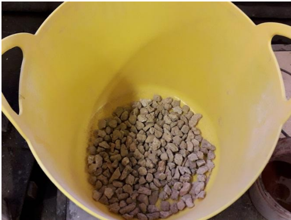
Fig. 5: Mixed concrete/mineral aggregate (16-20 mm) fraction
