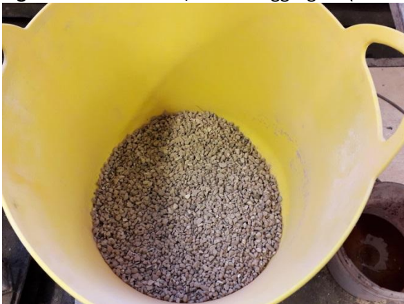
Fig. 6: Mixed concrete/mineral aggregate (8-16 mm) fraction
