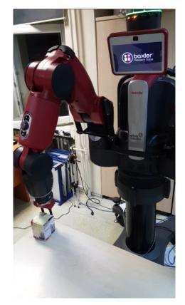
Fig. 1: Baxter robot pushing an object on table along a curved trajectory to a goal position.
