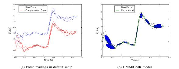
Fig. 2: (a) Raw and compensated force readings in x dimension. Three trajectories correspond to execution of the push action with object in default position initially. (b) The corresponding HMM model of the force trajectory with 10 hidden states. Mean and variances of hidden states represented by a univariate Gaussian distribution are shown by dark blue ellipses' center and radii.
