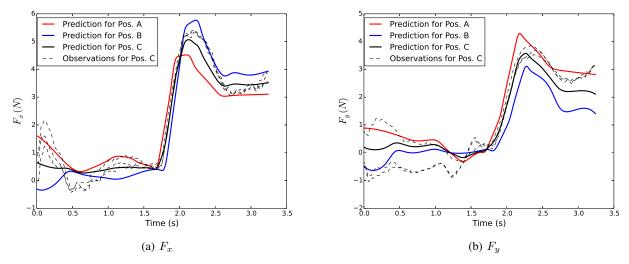
Fig. 6: Generalization of tactile feedback in (a) forces in x direction and (b) forces in y direction. Red line corresponds to forces when the wrist angle equals to 0.7 rad, Pos. A; blue line corresponds to forces when the wrist angle equals to 0.2 rad, Pos. B. Dashed lines represent forces of 3 demonstrations when the wrist angle equals to 0.45 rad, Pos. C. The green line corresponds to the GMR reproduction of these three demonstrations.
