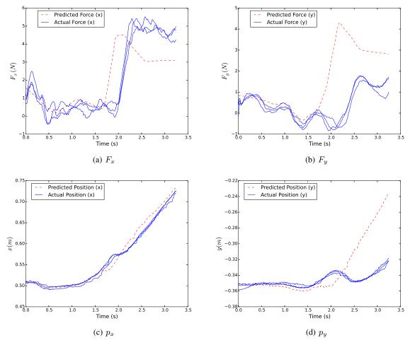
Fig. 3: This figure shows how the actual force feedback deviates from the predicted one (at around t = 1.7s), and how the position of the gripper adapts in response to this change.
