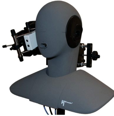
Figure 4.3 Dummy-head used in AIR dataset with the two-microphone mock-up clamped in the hand-held positioner.
