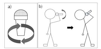
Figure 1: a)Circular motion of Voicon generates vibrato. b) Vocal performer can tilt the Voicon upward/downard to raise/lower the pitch.
