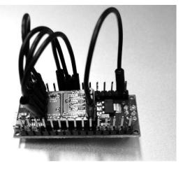
Figure 3: Arduino Nano with the tri-axial accelerometer.
