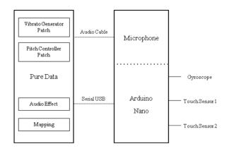
Figure 5: The internal components of Voicon.
