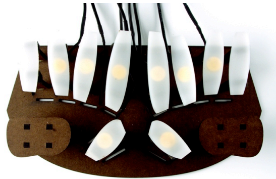
Figure 4. Prototype 2: Laser-cut from Masonite and acrylic plexi; Ten finger pads all made of acrylic plexi and arranged to match finger positions. Audio cables exit from the front of the instrument independently.
