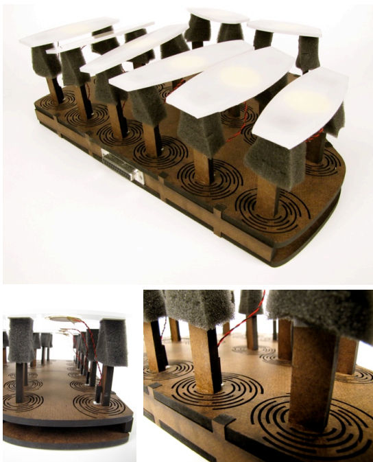
Figure 5. Prototype 3: Top: Eight finger pads, DB-25 connector carrying all eight balanced signals exists from front of instrument; larger finger pads for easier interaction; Bottom Left: audio cables from each microphone with JST connectors to enter the space between the base plates where they converge into the DB-25 connector; Bottom Right: better isolation vibration achieved with a series of concentric arcs around the base of each finger-pad
